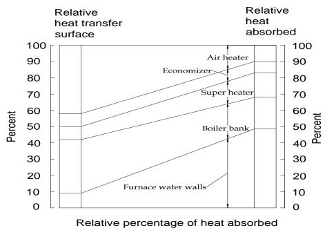
through heat transfer of bagasse fired boilers
